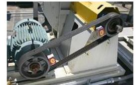
The Belt Hog from Peterson Alignment Tools Company makes it simple to align belts and pulleys. You won't have to remove the belts to make quick, accurate adjustments over distances of 6" to 20 feet. One person can accomplish an alignment with no training other than reading the short instruction manual.
