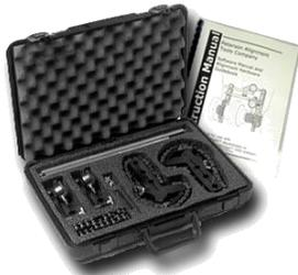
Like its partner above, the 30RA comes in its own rugged carrying case containing all of the hardware necessary to perform both radial and angular alignments in one quick step: two larger, high-quality aluminum mounting frames for higher reach and longer span, two top-quality dial indicators, two indicator mounting rods with swivel joints, and stainless steel mounting tubes ranging from 5 to 15 inches in length.
